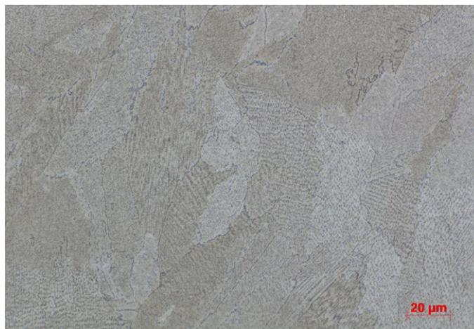
A family of nickel-based superalloy powders with chemistry similar to AMS 5662 bar material. Room temperature static properties of LB-PBF processed and heat treated material coupons have been shown to be comparable to those of AMS 5662.
