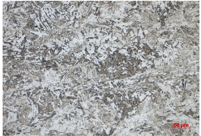
A family of martensitic, precipitation-hardening stainless steel powders with chemistry similar to AMS 5643. Room temperature static properties of LB-PBF processed and heat treated material coupons have been shown to be comparable to those of AMS 5643 in the H900 state.
