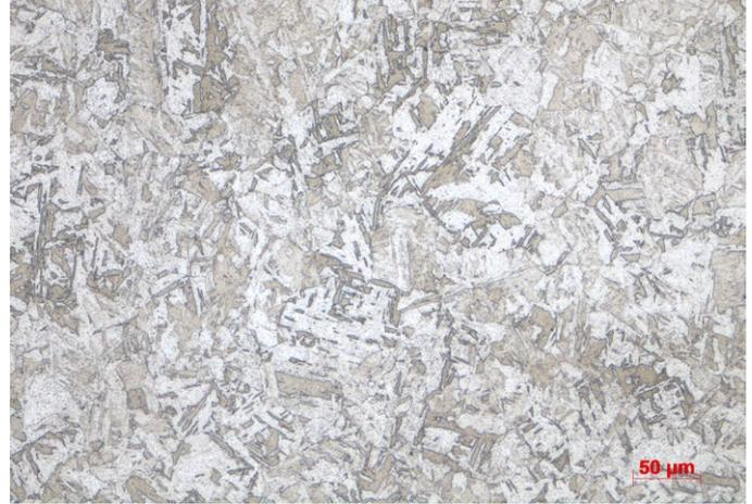
A family of martensitic, precipitation-hardening stainless steel alloy products with chemistry similar to AMS 5659. Room temperature static properties of LB-PBF processed and heat treated material coupons have been shown to be comparable to those of AMS 5659 in the H900 state.
