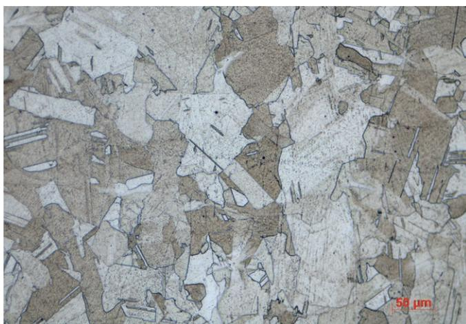
A nickel-based superalloy powder product with chemistry similar to AMS 5666 and Inconel 625 bar material. The material is optimized for producing additive manufactured components using Laser Powder Bed Fusion (LB-PBF).
