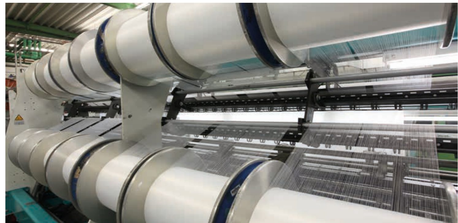
The warp knitting process requires extremely high yarn quality in order to guarantee an even fabric
