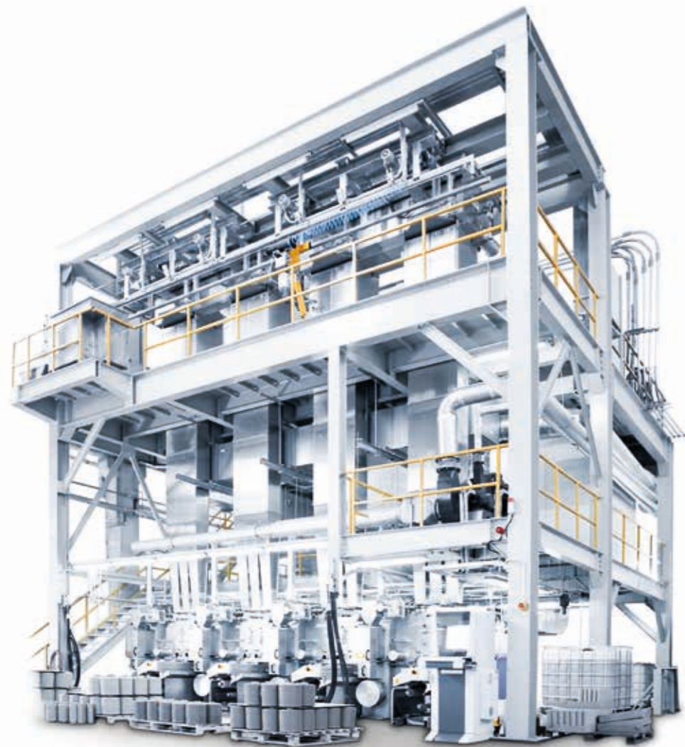
Oerlikon Neumag's BCF carpet yarn machine S+ also processes recycling polyester. In addition, the e-save certified machine consumes at 1850 dtex for example 17% less energy than its predecessor machine S5.
