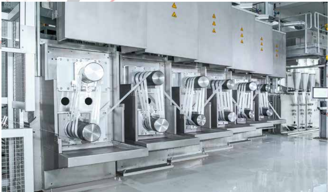
The Staple FORCE S 1100 spins, draws, crimps, cuts and bales in a single process step. Here, the fiber tow is drawn using godets in a highspeed process. Sets of godets positioned above each other form a stretch duo with its own hood.
