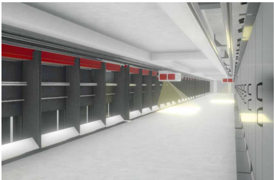
The wiping robot is suspended on a track system under the ceiling.
