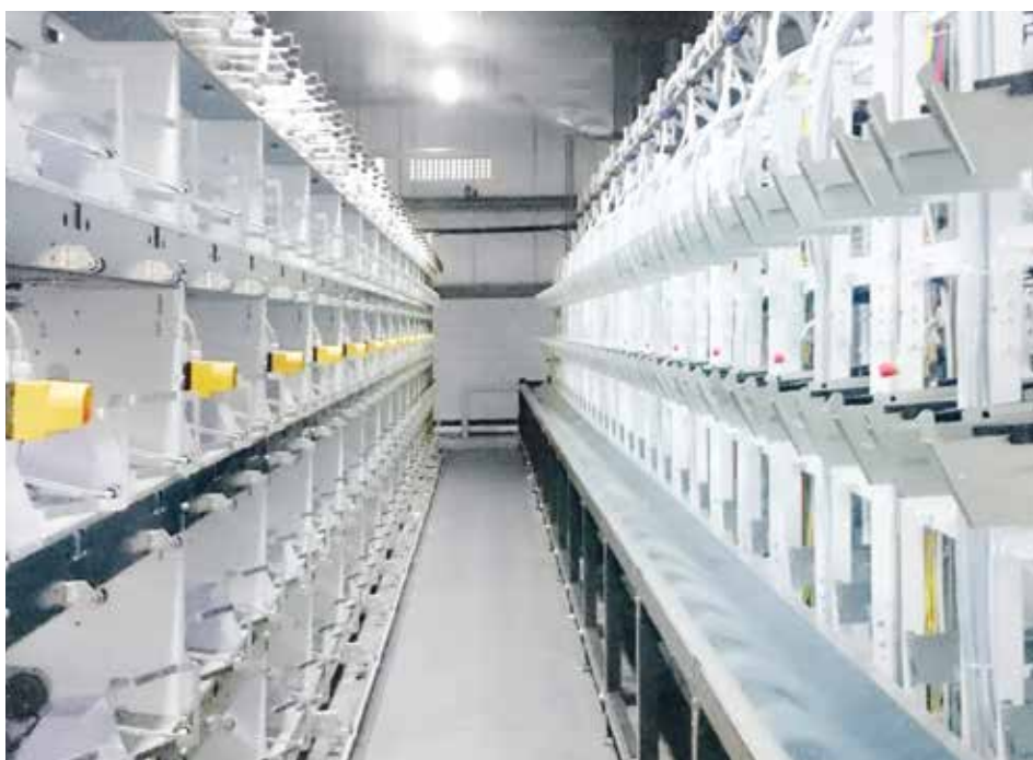
The economic way of tape yarn production: The automatic WinTape winder can run for up to 24 hours without operator at speeds of up to 800 m/min.
