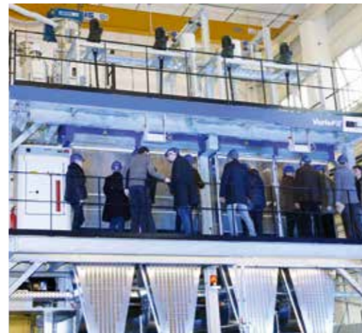
VarioFil R+ is the first POY spinning system that produces yarn directly from recycled flakes.
