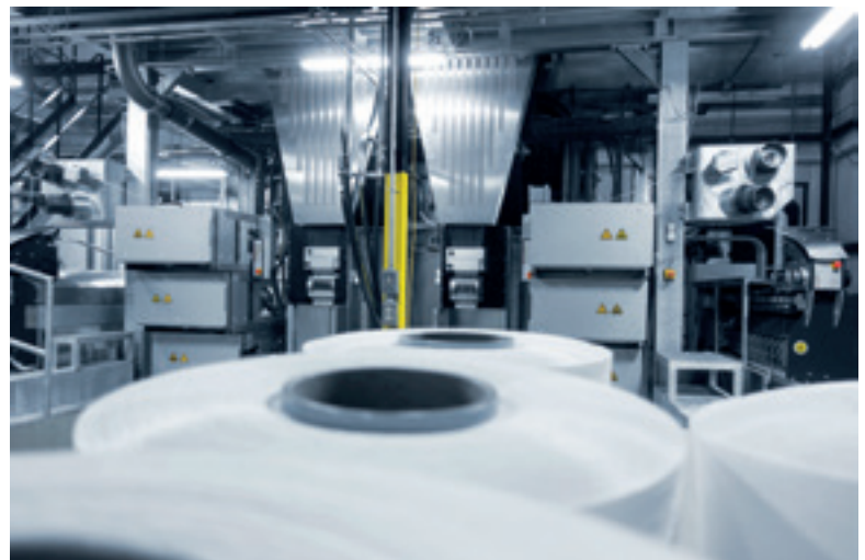
Barmag Brückner Engineering's (BBE) compact spinning line VarioFil processes polypropylene with WINGS technology.
