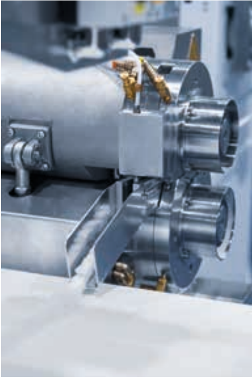
The crimper has been redesigned according to the stuffer box crimping principle.
